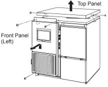
Top Panel: Remove the screws and lift off. Front Panel (Left): Remove the screws. Lift up and pull toward you.
